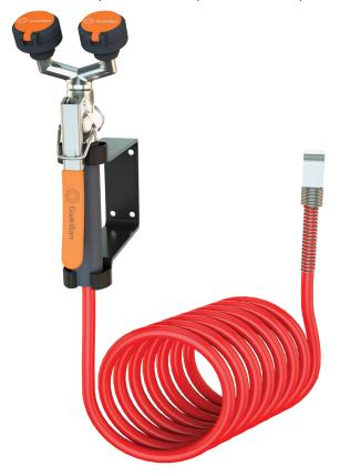
**Application:** Dual purpose eyewash/drench hose with 12' coiled hose for wall mounting. Unit meets the provisions of ANSI Z358.1-2014 as both an eyewash and a drench hose. Unit may be left in the mounting bracket for use as a fixed eyewash, leaving user's hands free. Alternatively, unit may be removed for use as a drench hose to rinse any part of user's eyes, face or body. 12' nylon retractable hose coils to eliminate trip hazard.
